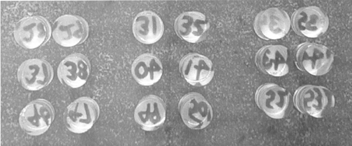
Figure 3 Workpieces ground with microstructured belts. The three rows show that excellent surface finish can be achieved with moderate abrasive particle size, moderate belt speed, and high material removal rate.
