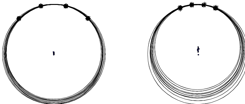
Figure 2: calculated LSQ-circles for diameter measurements, 2 different measurement strategies
