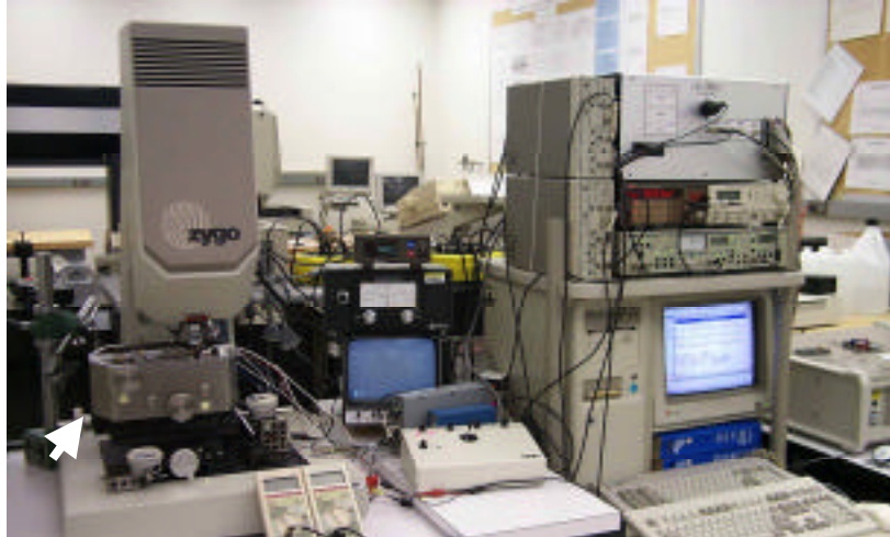
Figure 2 Photograph of the experimental setup for nanoindentation
