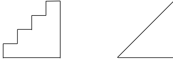
Figure 2. The staircase profile on the left is a binary approximation of the continuous profile on the right. The profile on the right is achievable using grayscale mastering. With binary masters, the steps on the staircase profile are reduced as the number of levels is increased; however the increased cost and the manufacturing inaccuracies can outweigh the efficiency improvements. For this reason, 4 to 8 level structures are typically used to approximate a blazed grating.
